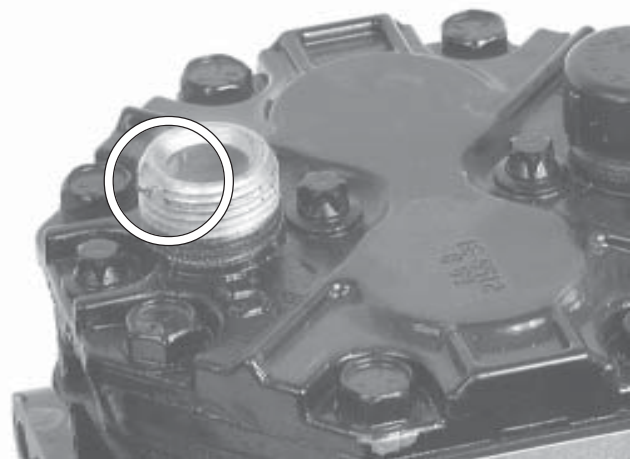
Dropped Compressor shown by the flat dent in threads
